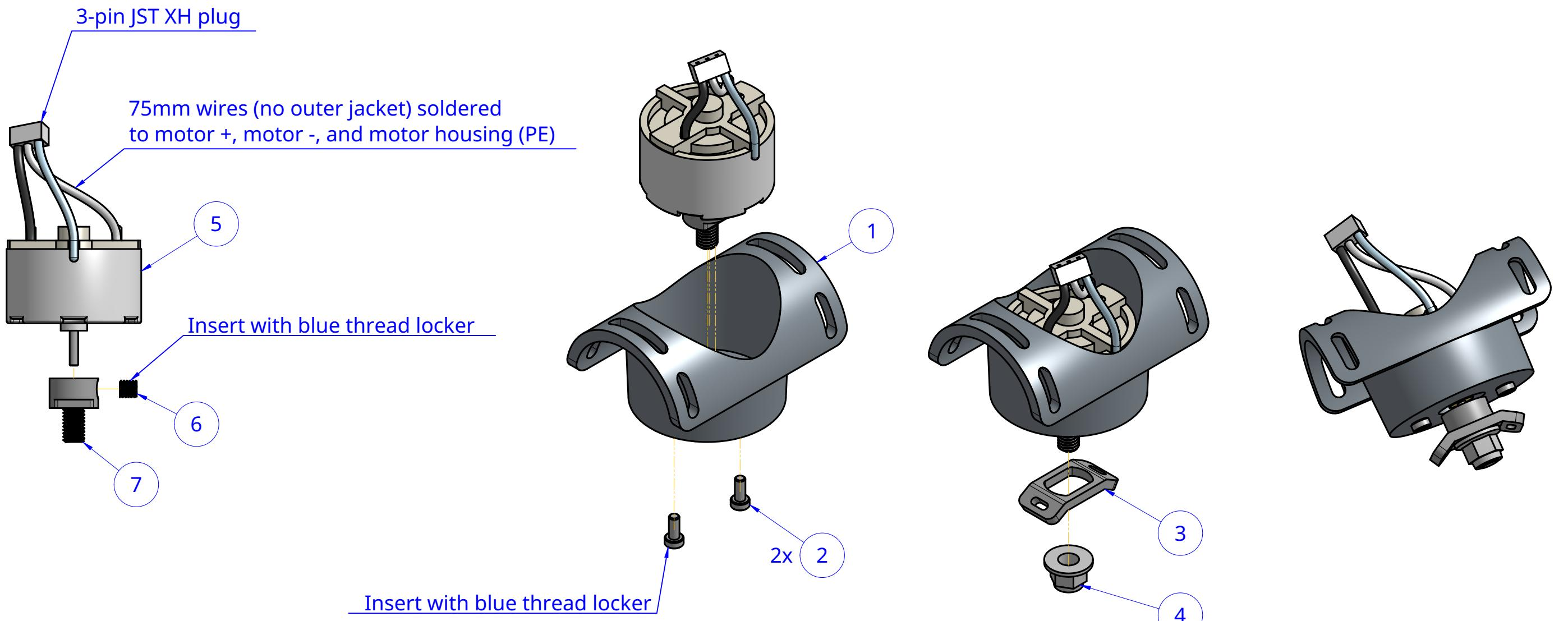
Pre-Assembled Rotary Tool Bottom Rev B
